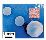
Micro/macroporous polycrystalline spheres of microporous titanosilicate umbite were prepared by hydrothermal synthesis without the use of organic structuring agents.
